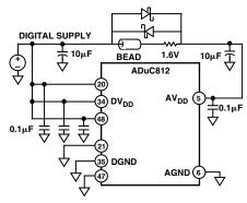
Figure 44. External Single-Supply Connections
